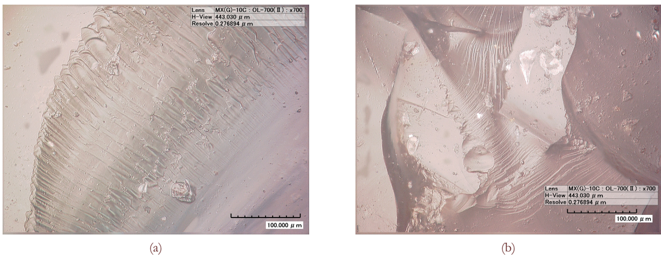
Figure 14: Fracture surface of quartz. Optical microscopy.
