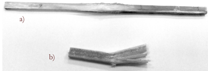
Figure 8: Failed unidirectional fiberglass (Direct "E" roving 0.7 - orthophthalic polyester resin 0.3) at three point bending tests on large (a) and small (b) bases.
