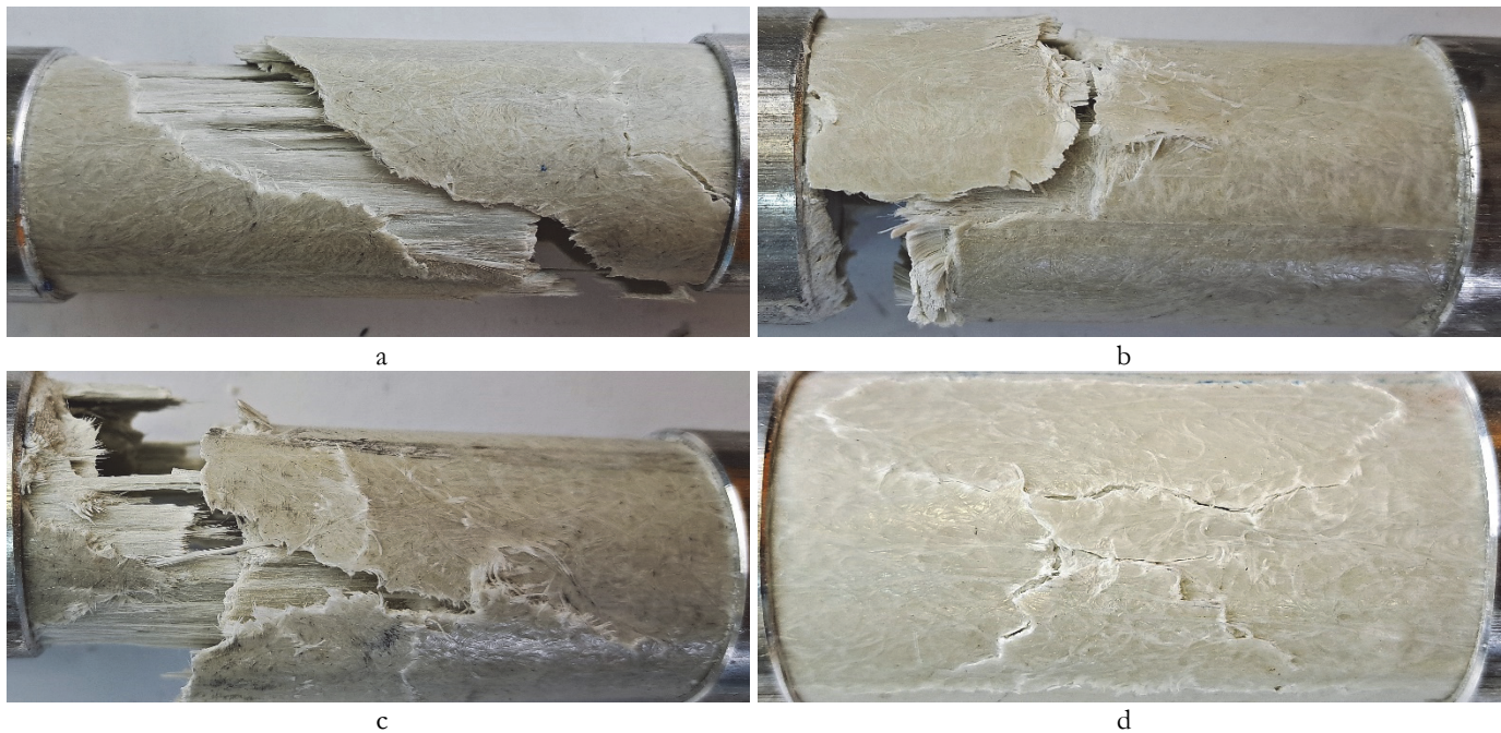
Figure 7: Images of specimens after cyclic: tension-tension (a); compression-compression (b); tension-compression (c); torsion (d).
