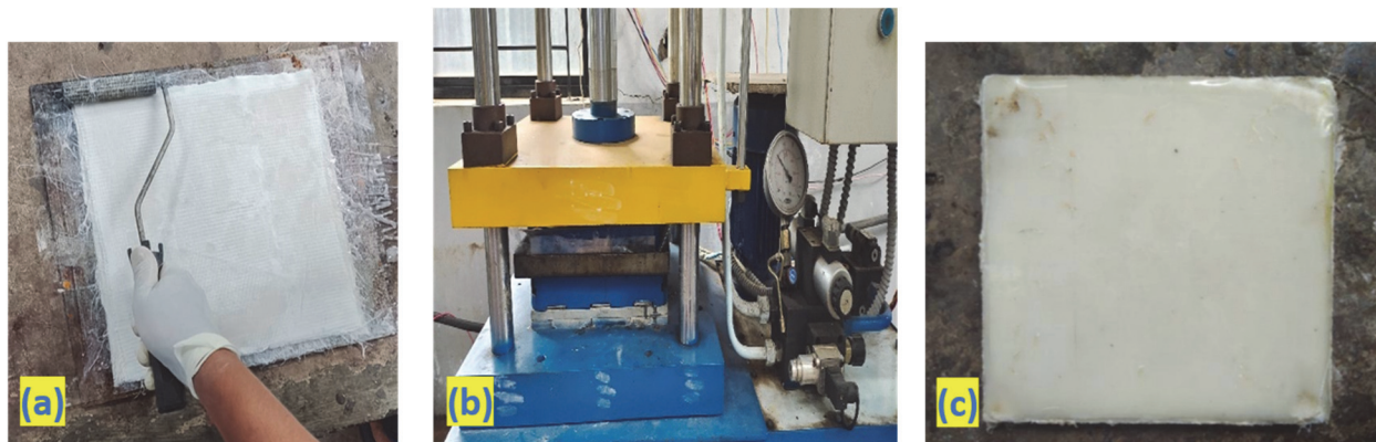
Figure 2: (a-b) Fabrication process (c) Composite plate.
