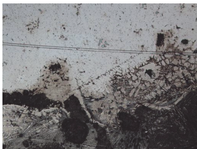
Etched section of the fusion line and the heat affected zone with hard martensitic and ledeburitic microstructures
