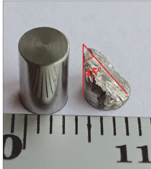
Figure 5: Specimen before and after failure (HEA52).
