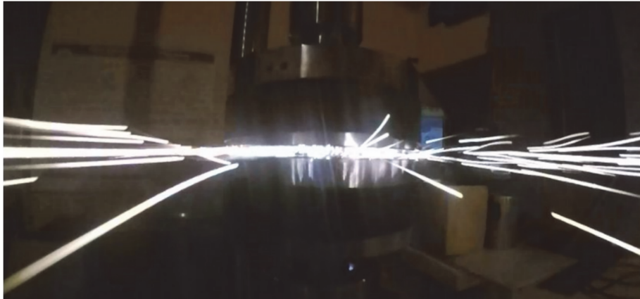
Figure 3: Explosion of HEA55 specimen and ignition of its particles (high-speed shooting, 240 fps).
