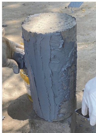
(b) First layer of adhesive
