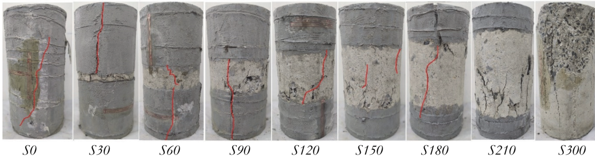
Figure 10: Failure mode of cylinders.
