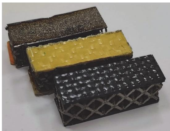
Figure 2: Titanium, AFRP and PW-CFRP short beam hybrid specimens, from left to right.
