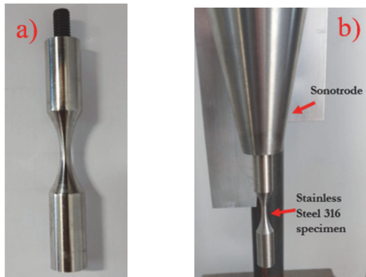
Figure 3: a) Machined specimen, and b) Specimen mounted in the ultrasonic machine.
