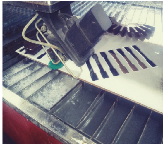
Figure 3: Cutting the specimens using the water jet process.
