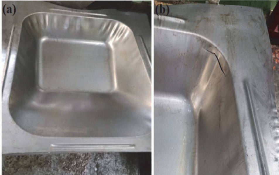
Figure 1: Appearance of rupture and wrinkling in extra-deep drawing of wheelbarrow trays.
