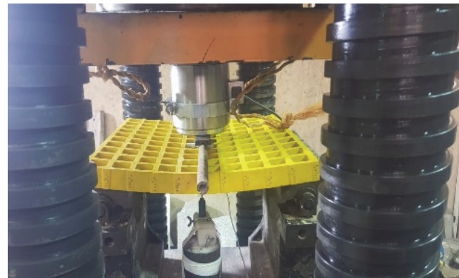
Figure 6: Load bearing test set up for GFRP gratings specimens
