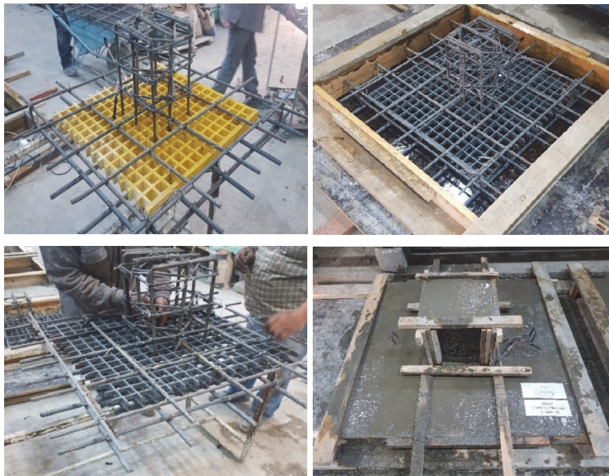
Figure 2: Tested specimen's preparation, reinforcement, and cast
