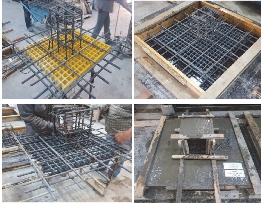
Figure 2: Tested specimen's preparation, reinforcement, and cast.
