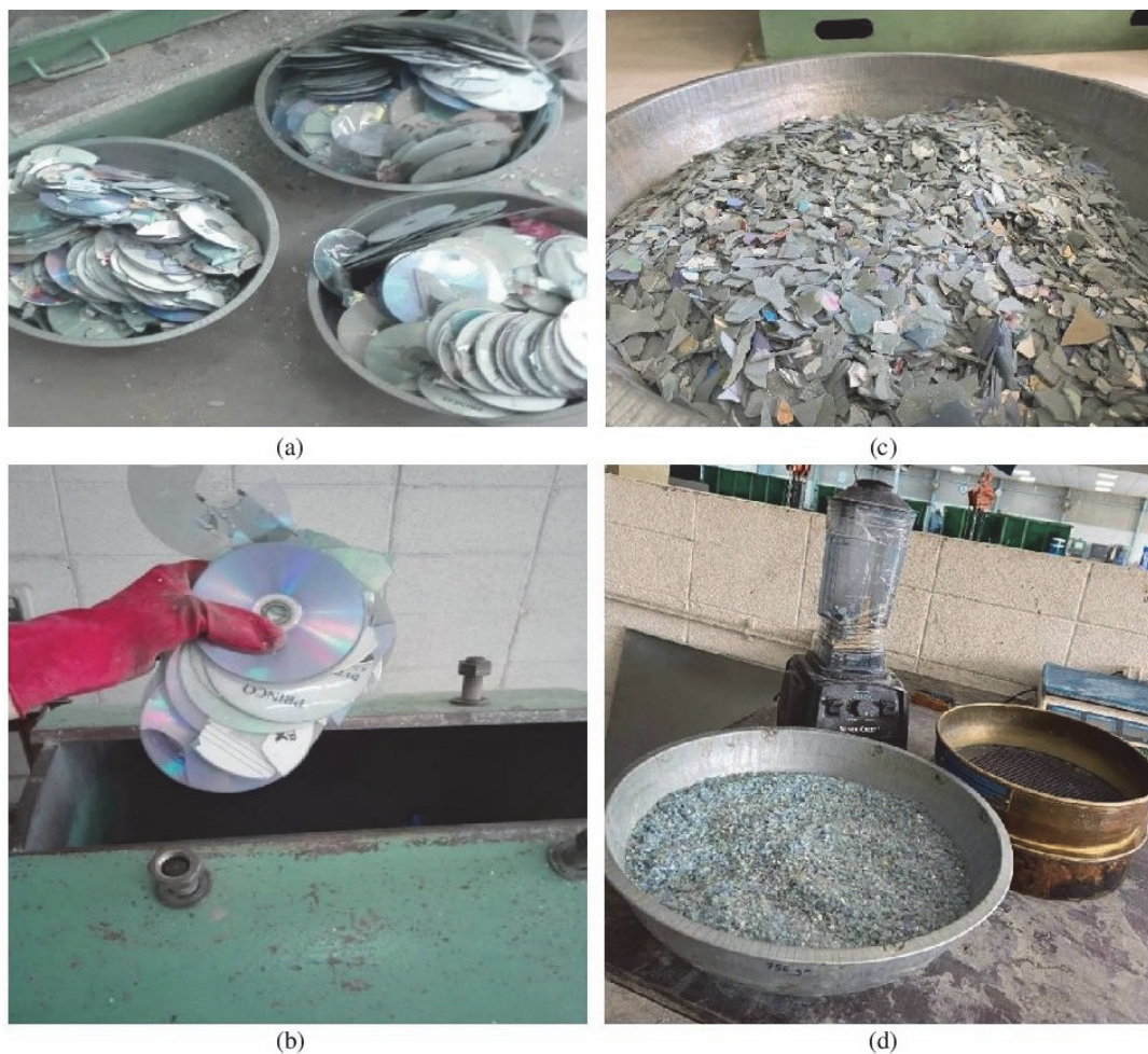
Figure 2: Disc shredding procedures: (a) Disc collection, (b) Crushing discs by Los Angeles machine, (c) Disc particle sizes after Los Angeles machine, and (d) A domestic mixer and sieving to produce the desired particle size.
