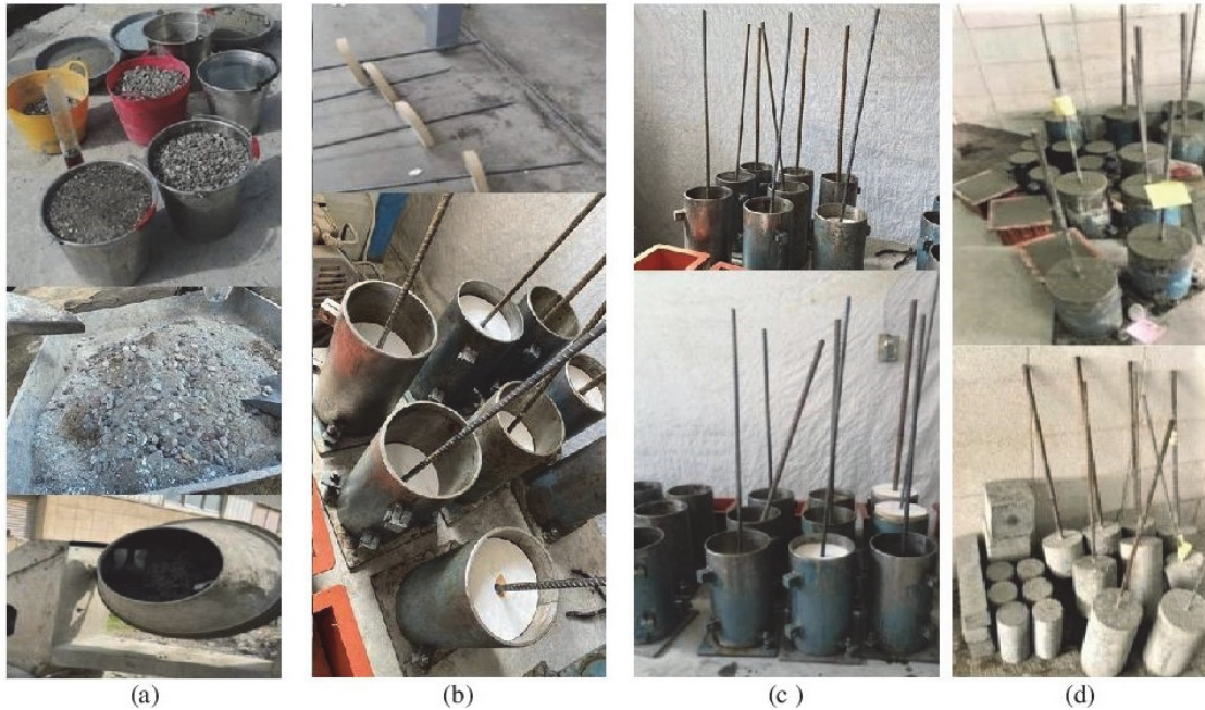
Figure 3: Casting the specimens: (a) Weighing the ingredients and mixing with mixer, (b) Positioning and fixing the steel bars with circular piece of wood inside the molds, (c) Putting the molds on the vibrating table, and (d) Casting and storing the specimens at ambient temperature.
