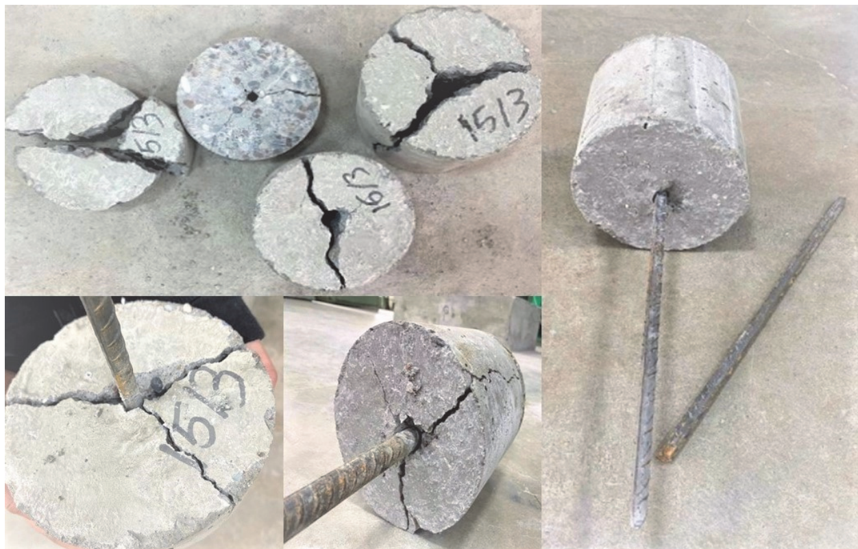
Figure 7: Failure modes of pull-out specimens.
