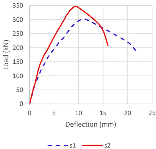
Figure 18: Load versus mid-span deflection for flat slab subjected to 4 and 6 strands for “control specimens”, which without any openings, (S1 and S2).
