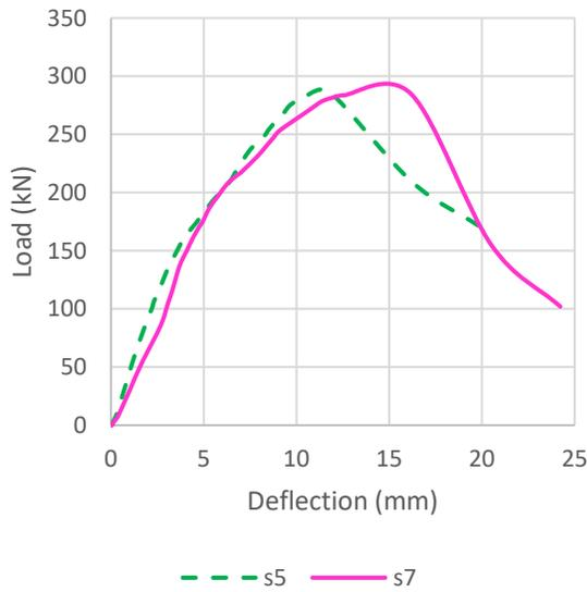
Figure 20: Load versus mid-span deflection for flat slab subjected to 6 strands specimens “specimens with openings either before or after Casting” (S5 and S7).
