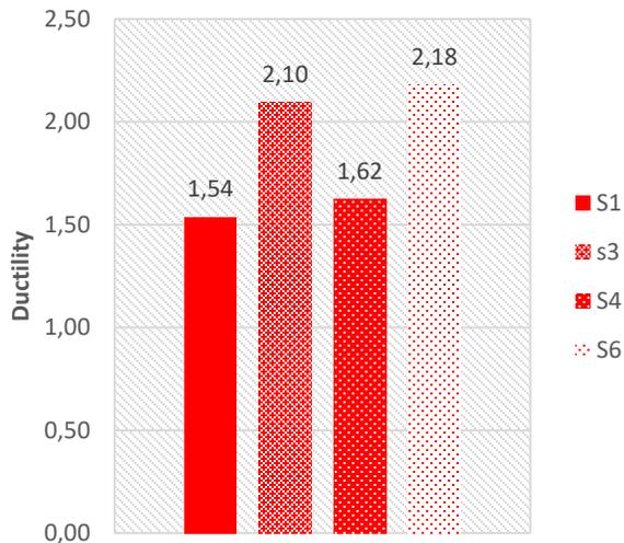
Figure 23: Ductility induced from 4 strands post-tensioned flat slab.
