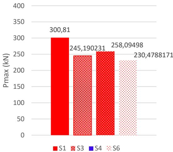
Figure 14: Load comparisons between control Specimen(S1) and specimens with openings subjected to 4 strands
