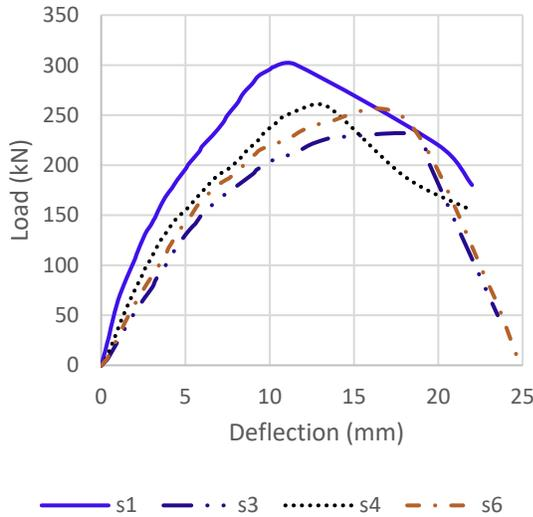
Figure 12: Load versus mid-span deflection for flat slab subjected to 4 strands, for control specimen (S1) and specimens with openings.
