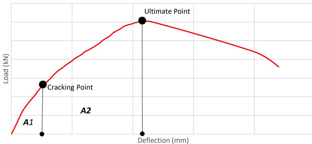
Figure 28: Indication for Calculating the Energy absorbed from Area under curve
