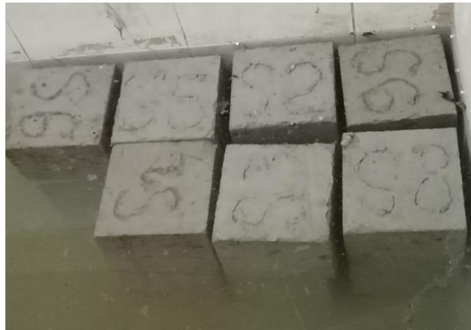
Figure 4: Standard cubes (150 x 150 x 150 mm), while immersed in water.
