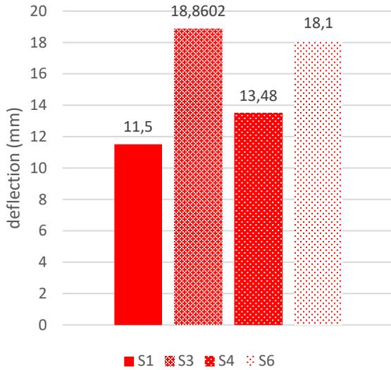
Figure 16: Mid-span deflection comparisons between control specimen(S1) and specimens with openings subjected to 4 strands.
