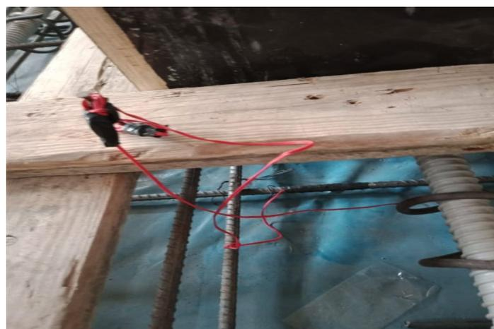
Figure 32: Strain Gauges it was installed on a slab reinforcement.
