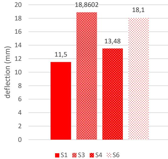
Figure 17: Mid-span deflection comparisons between control specimen(S2) and specimens with openings subjected to 6 strands.
