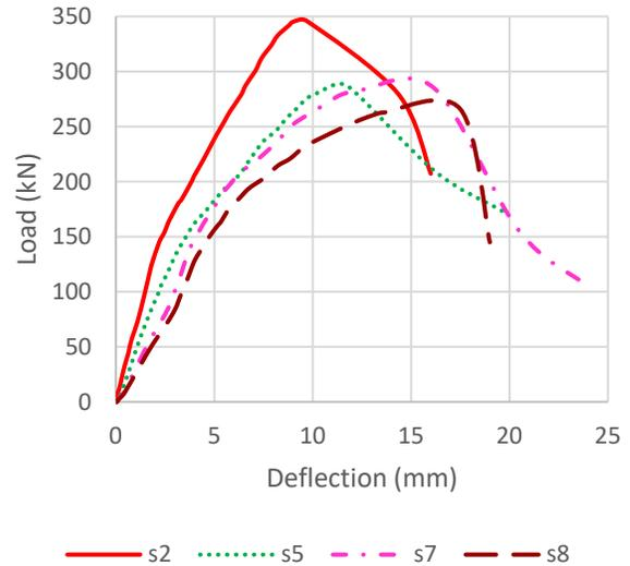
Figure 13: Load versus mid-span deflection for flat slab subjected to 6 strands, for control Specimen and specimens with openings.
