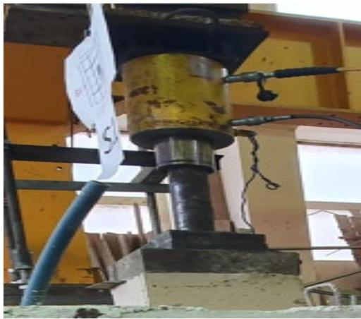
Figure 10: A metal plate between the jack of the loading machine and the concrete.
