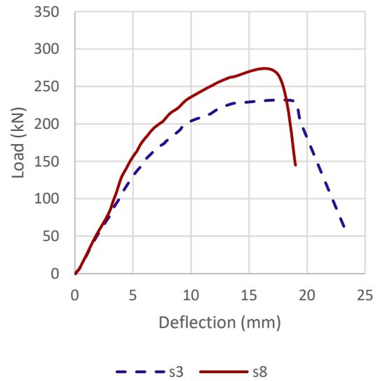
Figure 21: Load versus mid-span deflection for flat slab specimens with openings subjected to 4 strands, either before or after Cutting the Strands, (S3 and S8).
