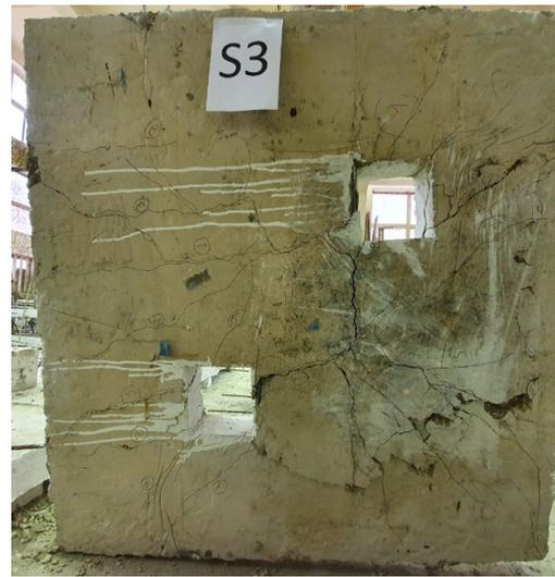
Figure 35: Punching failure surfaces of post tensioned flat slab Openings, (S3).
