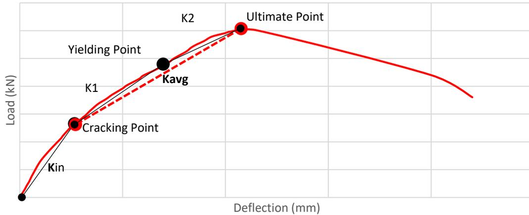
Figure 25: Indication for Stiffness of flat slab subjected to post-tensioned strands.
