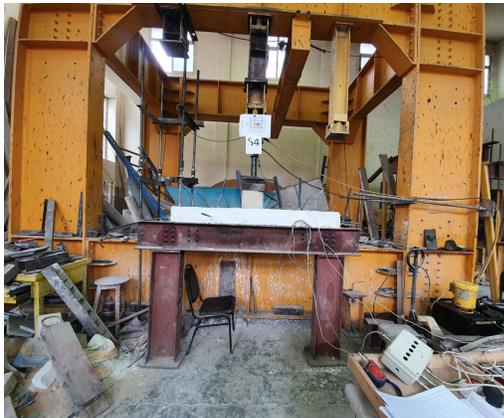
Figure 8: Test Setup for the loading machine on the slab.
