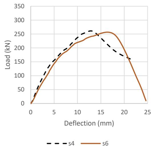
Figure 19: Load versus mid-span deflection for flat slab subjected to 4 strands specimens “specimens with openings either before or after Casting” (S4 and S6).
