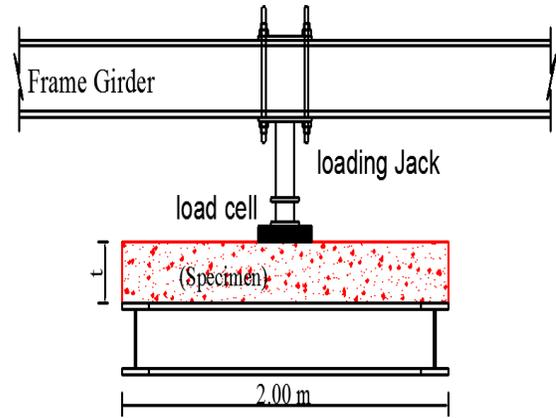
Figure 9: Illustration for the loading machine
