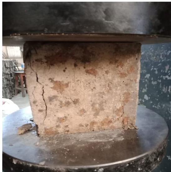
Figure 5: The shape of the cracks in the test cubes on the crushing machine.
