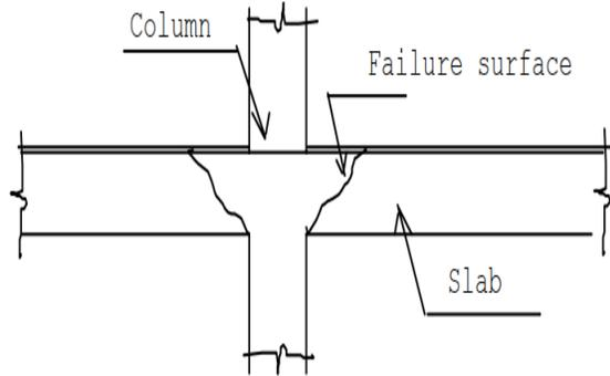
Figure 34: An illustration for Punching failure surfaces of tensioned flat slab.
