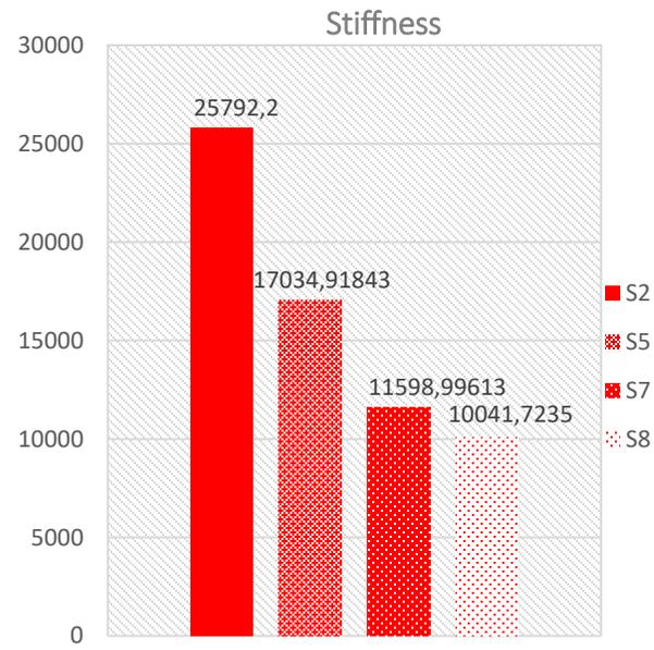
Figure 26: Stiffness induced from 4 strands post-tensioned flat slab.
