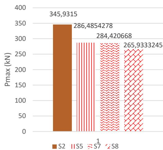
Figure 15: Load comparisons between control specimen(S2) and specimens with openings subjected to 6 strands.
