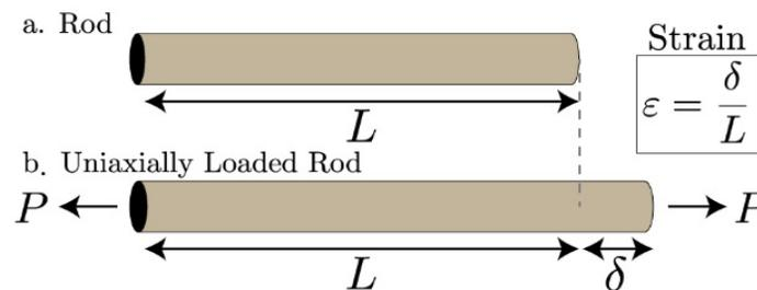
Figure 31: Strain mechanism.
