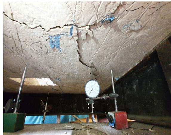
Figure 11: LVDT to measure slab deflections.
