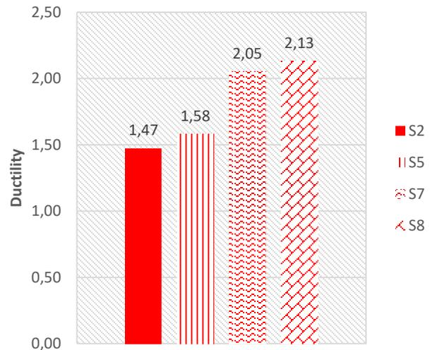
Figure 24: Ductility induced from 6 strands post-tensioned flat slab.
