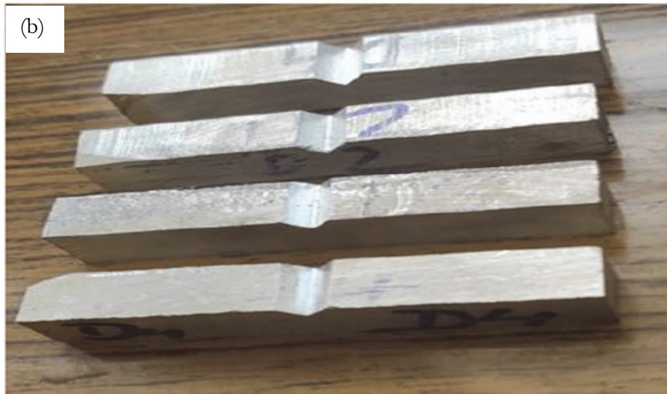
Figure 3: (a) Geometry and (b) Prepared Charpy V-notch specimens.
