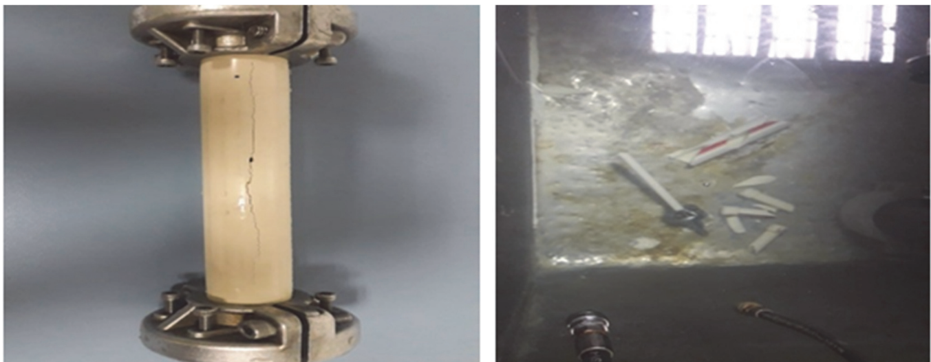
Figure 6: Breaking form of chlorinated PVC pipe.
