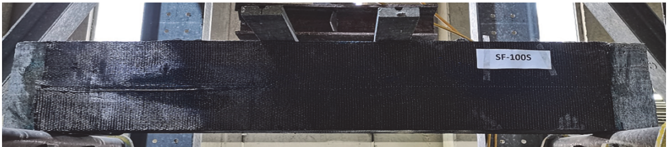
Figure 6: Full-height U-wrapping CFRP sheets and subjected to 100% of the damage.
