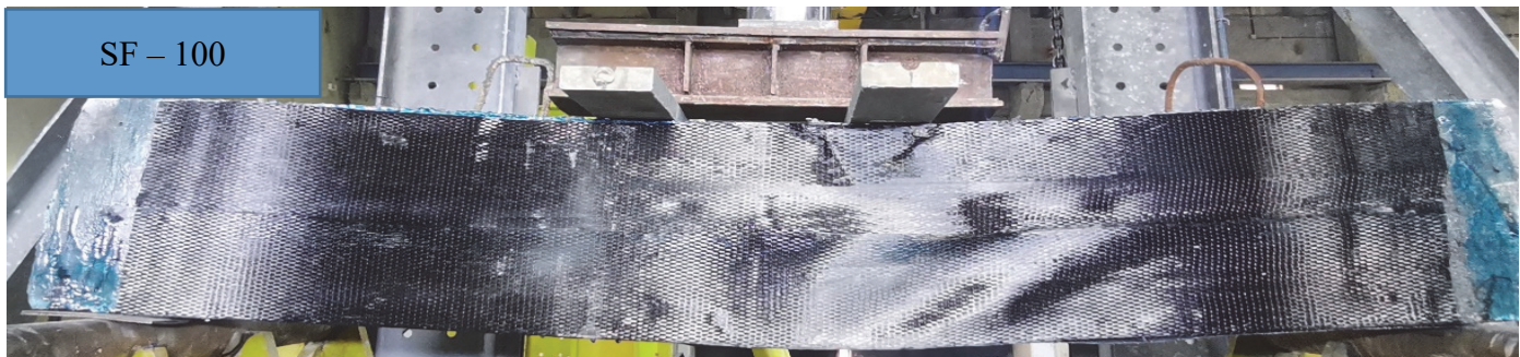
Figure 14: The mode of failure beam specimen (SF - 100).
