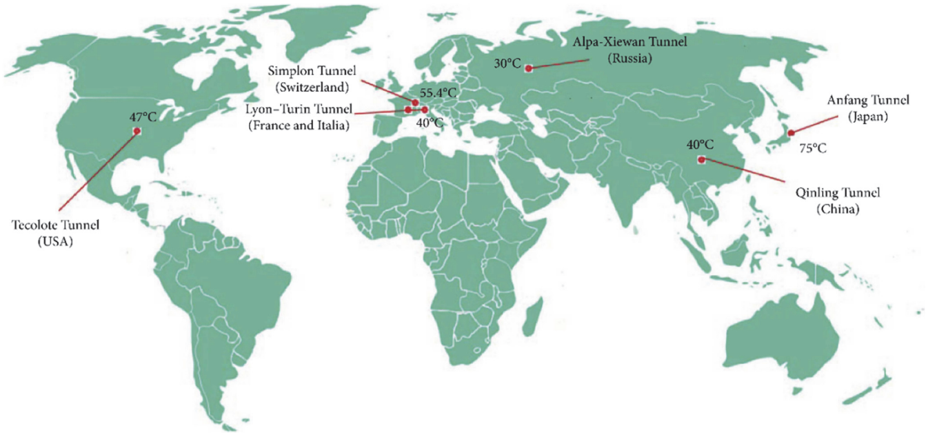
Figure 14: A view of geothermal extent in some tunnels in the world (Data from [119]).
