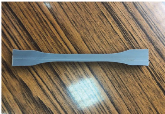
Figure 3: The CPVC specimen.
