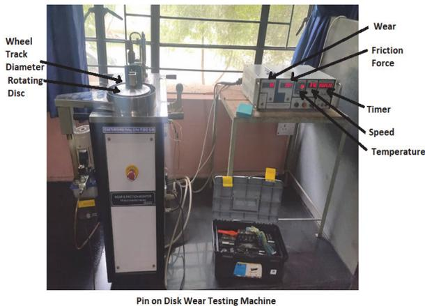
Pin on Disk Wear Testing Machine
