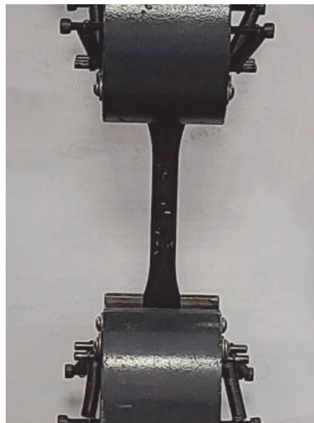
Figure 11: Test setup for specimens on SANTAM universal tension-compression testing machine.
