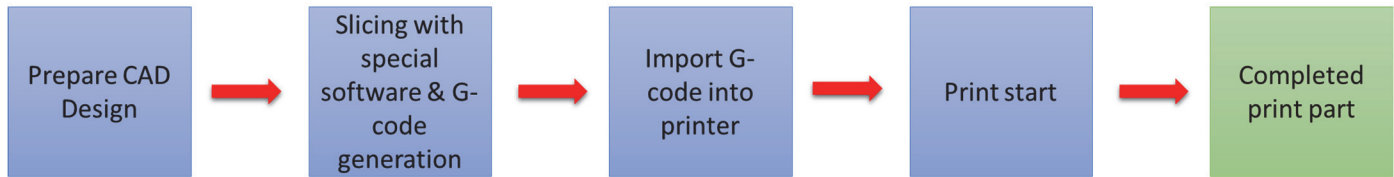
Figure 6: simplified process flowchart of FDM.
