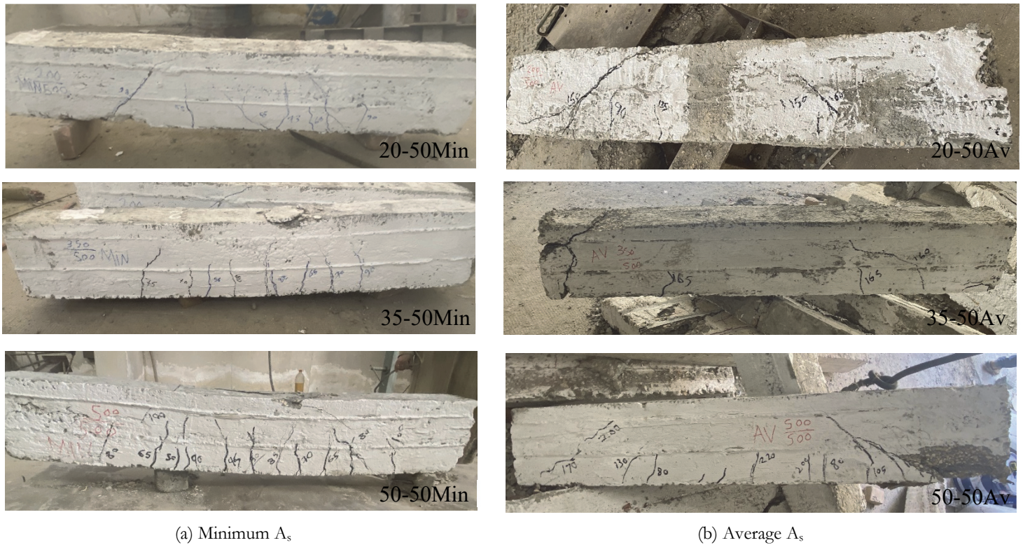
Figure 13: Crack pattern using concrete strength 50 MPa in tension zone and variation in Compression zone.
