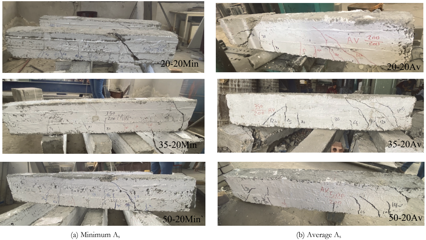
Figure 7: Crack pattern using concrete strength 20 MPa in tension zone and variation in Compression zone.
