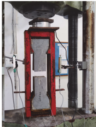
Figure 18: SSWM-Concrete Bond test failure of specimen.
