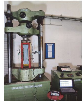
Figure 17: Experimental test setup for bond test.
