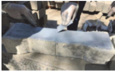
Figure 15: Preparation of dumbbell specimen for bond test.
