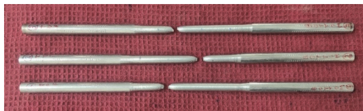
Figure 7: Failure of stainless-steel rod specimens.
