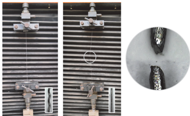
Figure 9: Tensile Test of Stainless Steel Wire and failure of wire.
