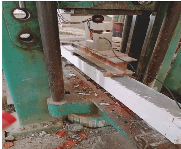
Figure 9: Four points loading applied to beam specimens.
