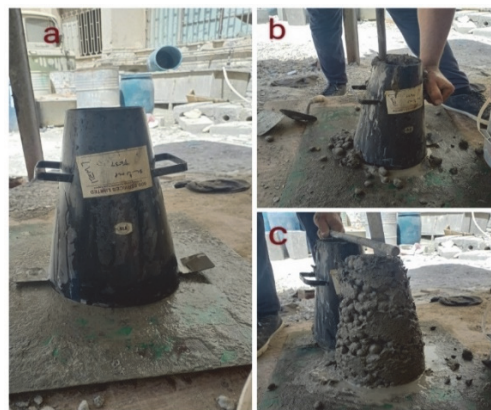
Figure 6: Steps of slump cone test.
