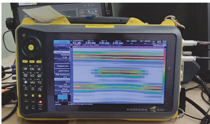
Figure 2: The ultrasonic flaw detector Harfang Veo 16-64 with a screen showing the "glueline defects" (a), and sensor on PAA 32 scanning defect in the sample (b)
