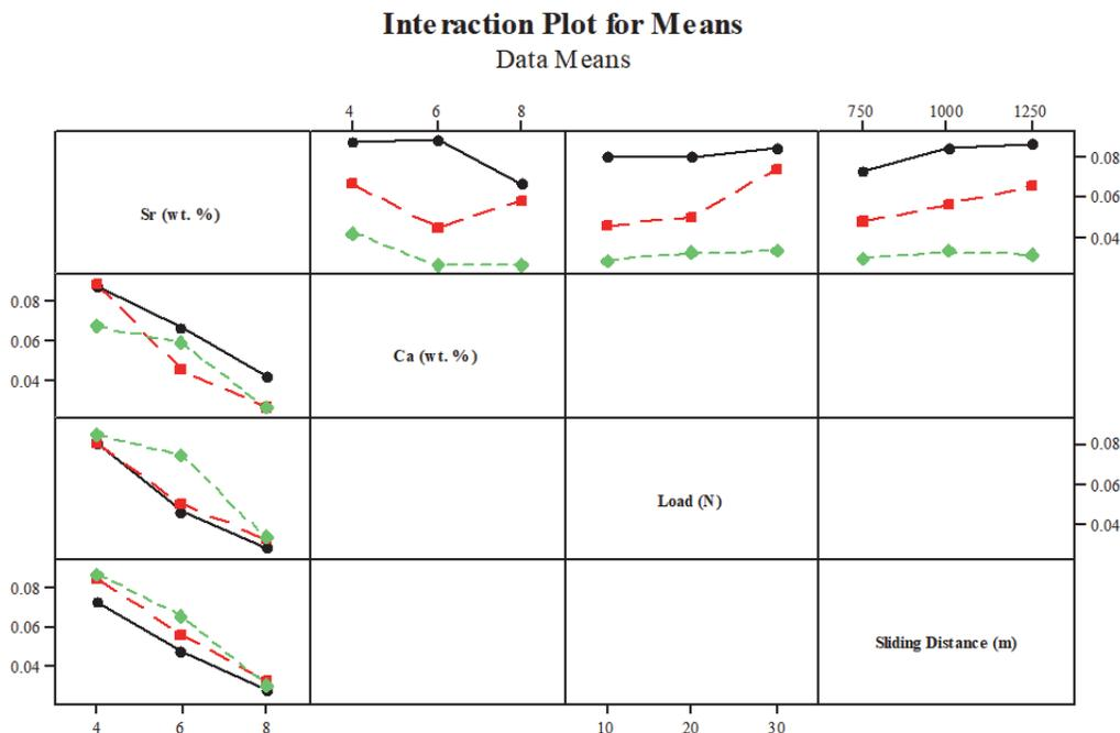
Figure 5: Interaction plots for wear loss.
