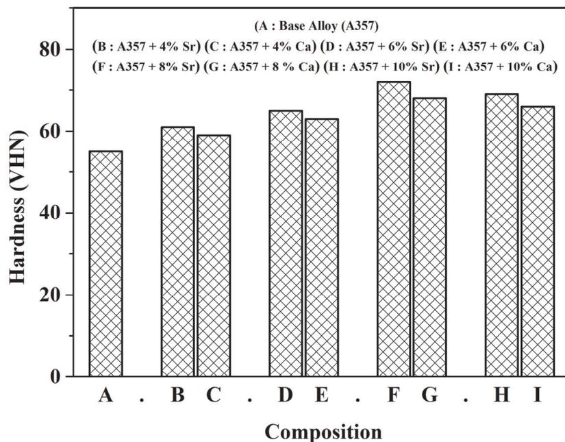
Figure 2: Hardness of A357 and varying wt. % of Sr and Ca
