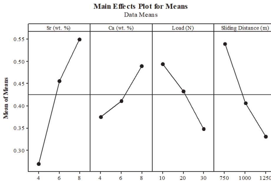
Figure 4: Effect of varying factor on COF.
