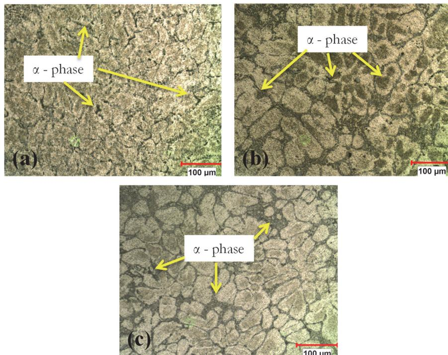
Figure 1. Microstructure images of (a) A357 (b) A357+Sr (c) A357+Ca
