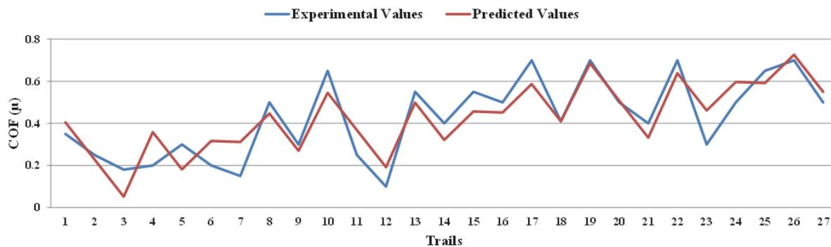
Figure 10: Comparison between experimental v/s. predicted values for COF.
