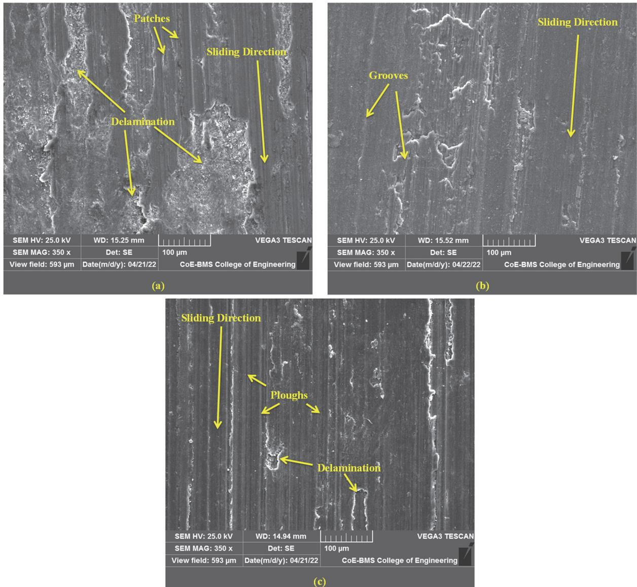
Figure 11: Worn-out surface morphology of (a) A357, (b) A357+Sr, and (c) A357+Ca.
