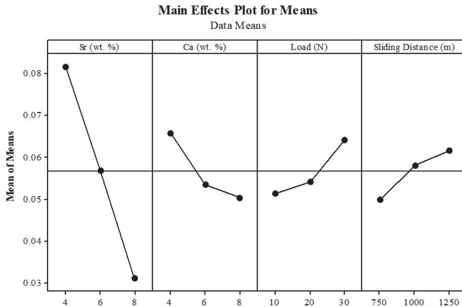
Figure 3: Effect of varying factor on wear loss.
