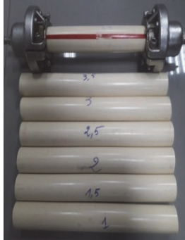
Figure 2: CPVC notched specimens at different depths.
