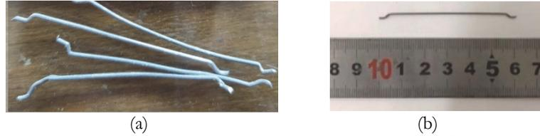
Figure 1: Hooked-end steel fiber. a) steel fiber set, b) fiber Dimension.
