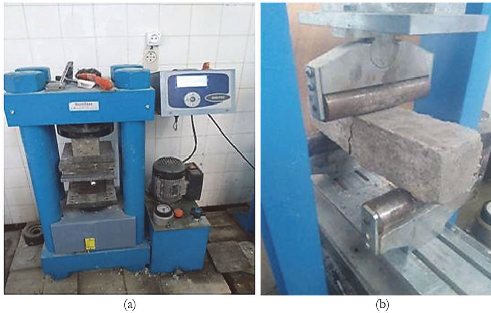
Figure 11: Hydraulics presses: (a) compression test and (b) three points bending test.
