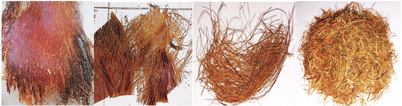
Figure 3: Preparation of date palm fibers mesh.
