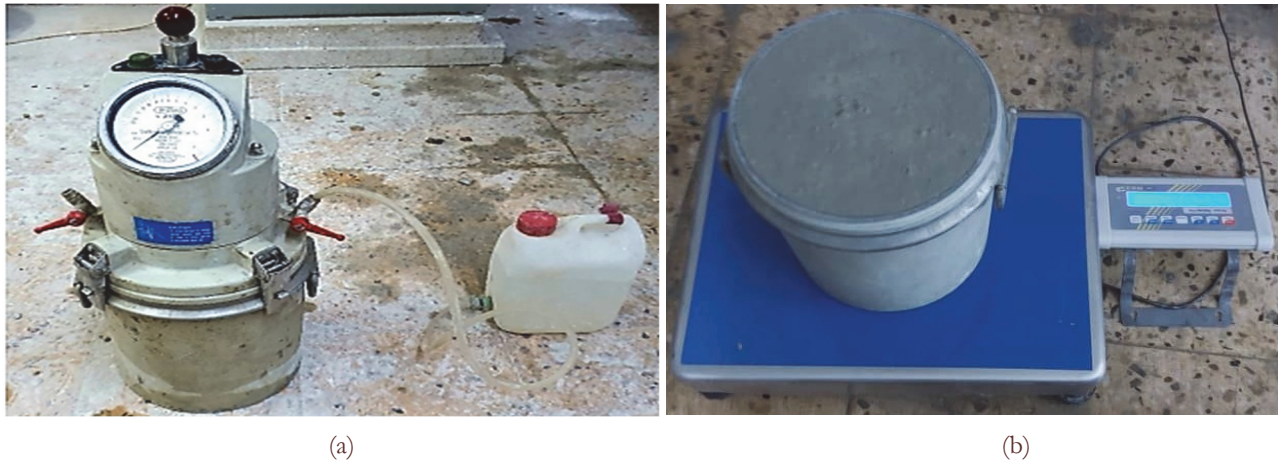
Figure 10: (a) determination of the entrained air with aerometer and (b) measure of concrete density in the fresh state.
