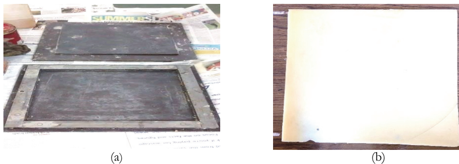
Figure 1: (a) Molds used for composite sheet preparation (b) Prepared epoxy sheet
