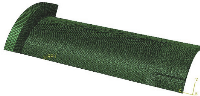
Figure 5: Finite element model with fine mesh of 0.82 mm element size.
