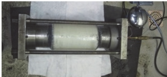
Figure 1: Repaired wall loss defect pipeline specimen for Hydrostatic test.
