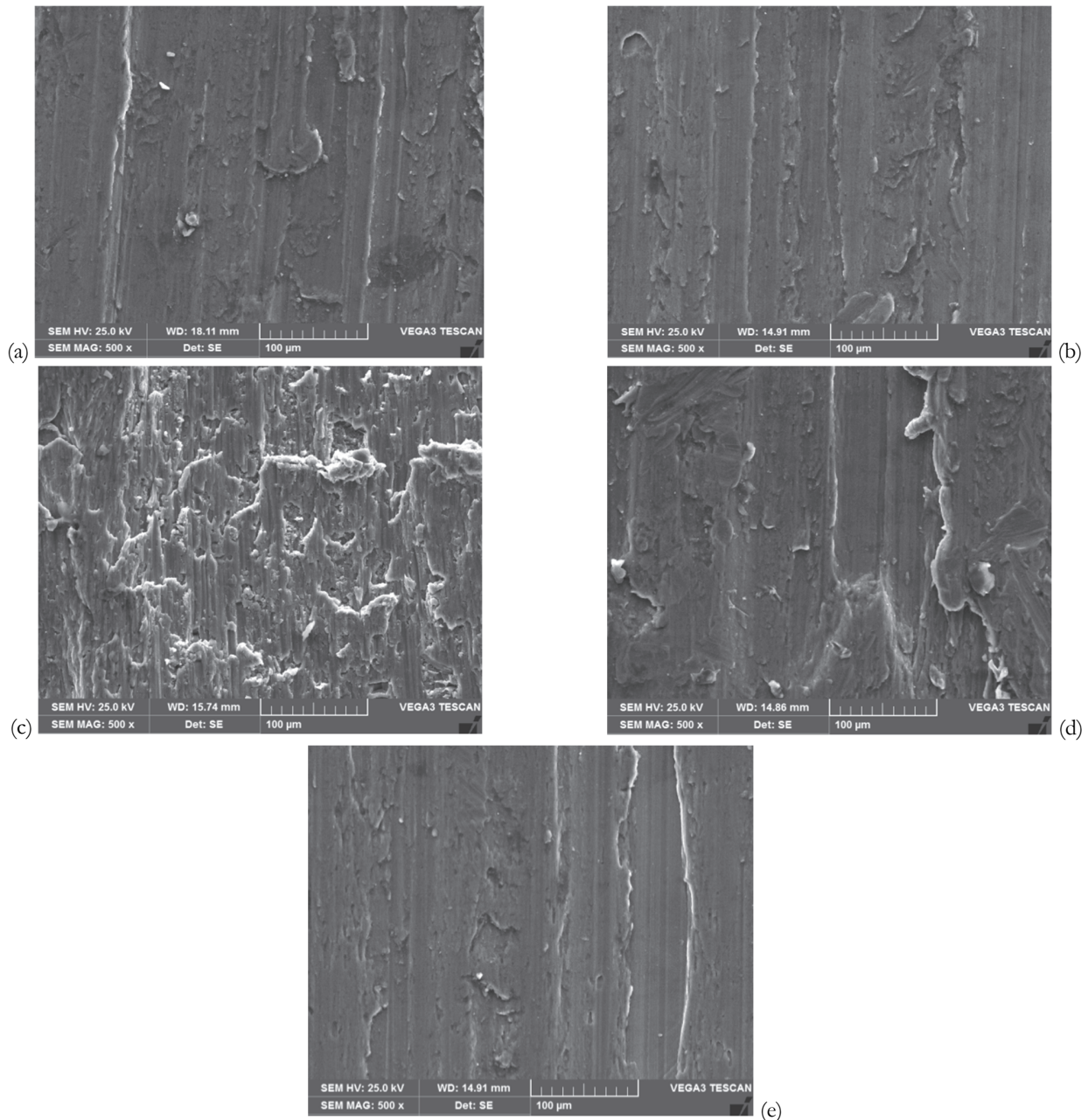
Figure 20: (a-e) Worn surfaces SEM micrographs of (a) Al2618 Alloy (b) Al2618-2 wt. % B 4 C (c) Al2618-4 wt. % B 4 C (d) Al2618-6 wt. % B 4 C (e) Al2618-8 wt. % B 4 C composites with 63 micron particles.
