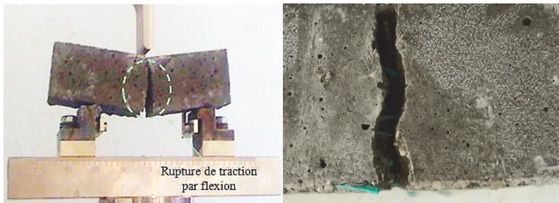
Figure 13: Failure mode of control sand concretes with 2% PET PB after the three point bending test.
