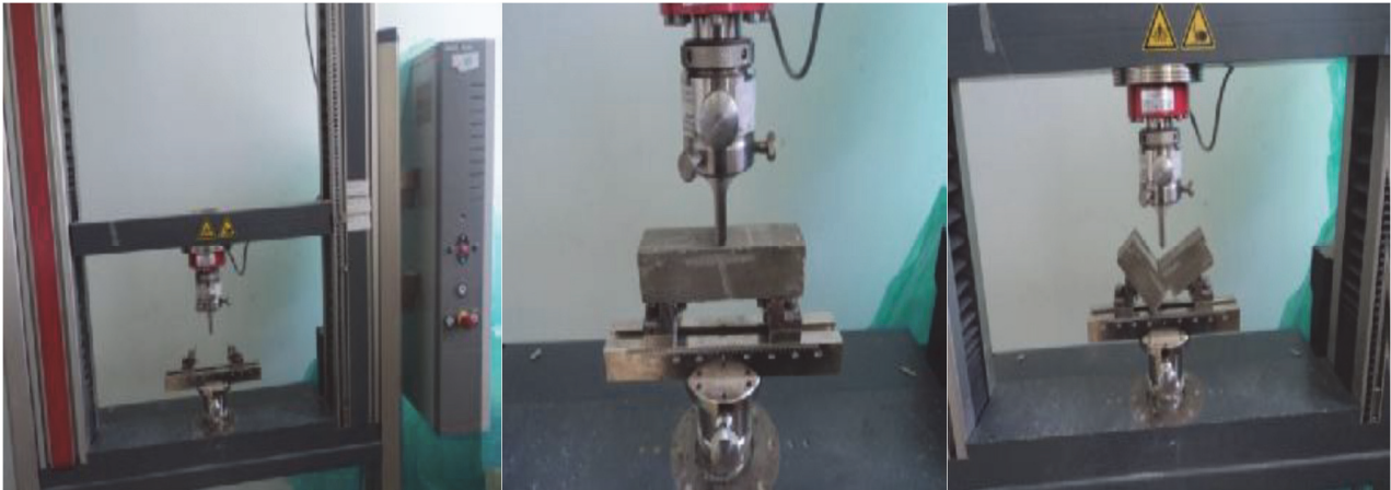
Figure 8: Bending tensile test on concrete specimens.
