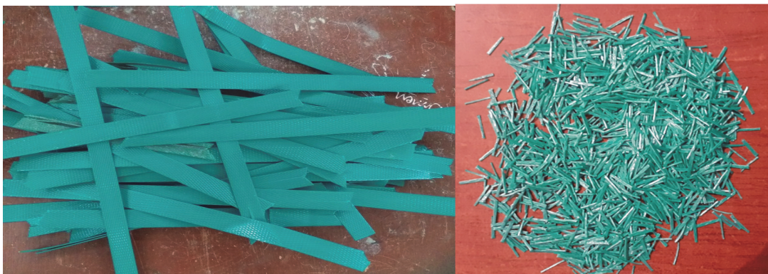
Figure 3: Optical photo of polyethylene terephthalate (PET) packaging belts.
