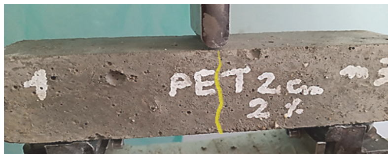
Figure 14: The failure mode of sand concretes with 2%PET after the three point bending test.
