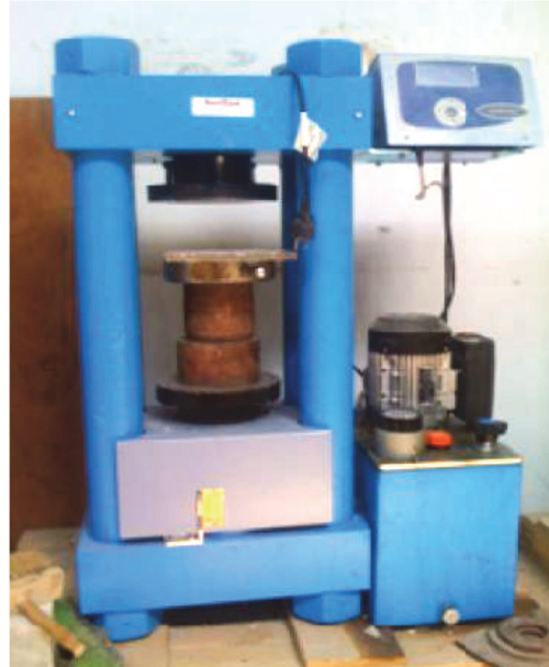
Figure 10: Compression test device.
