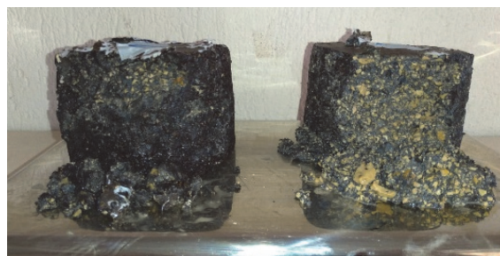
Figure 7: Samples prepared by using bituminous binder modified with 5% CDEA and 0.1% yarn waste fibers, after conditioning.
