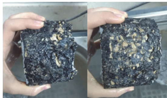
Figure 4: Sample prepared by using bituminous binder modified with 5% CDEA, after conditioning.
