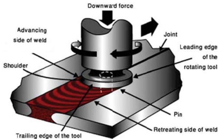
Figure 1: Schematic diagram of the FSW process.
