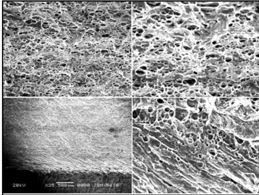
Figure 10: SEM images of tensile fracture surface of 6061-6082 at 62mm/min.
