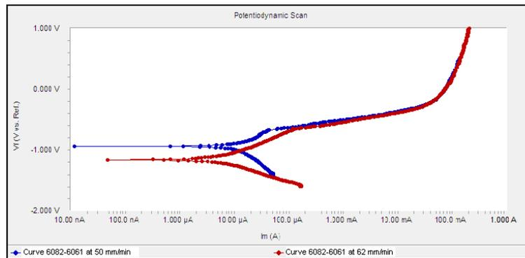
Figure 12: Polarization curves of AA6082-AA6061 at 50-62 mm/min.
