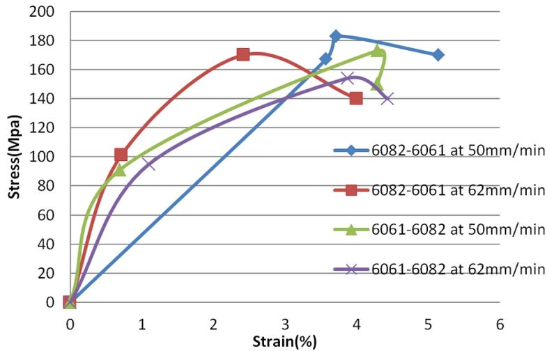
Figure 3: Stress-Strain curves for dissimilar alloys AA6082-AA6061.
