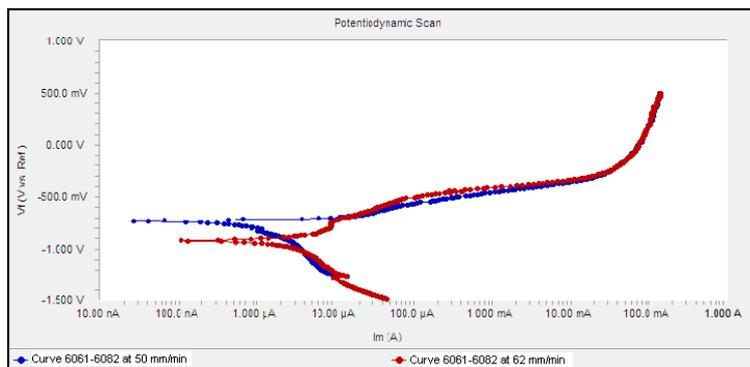
Figure 13: Polarization curves of AA6061-AA6082 at 50-62 mm/min
