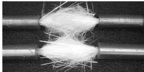
Figure 6: Failed unidirectional fiberglass (Direct "E" roving 0.7 - orthophthalic polyester resin 0.3) specimens after uniaxial tensile tests.
