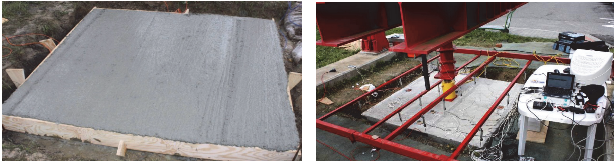
Figure 1: Casting and loading test of fibre-concrete slab.
