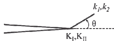
Figure 3: Inclusion of a small virtual crack emerging from the crack tip of a pre-existing crack.
