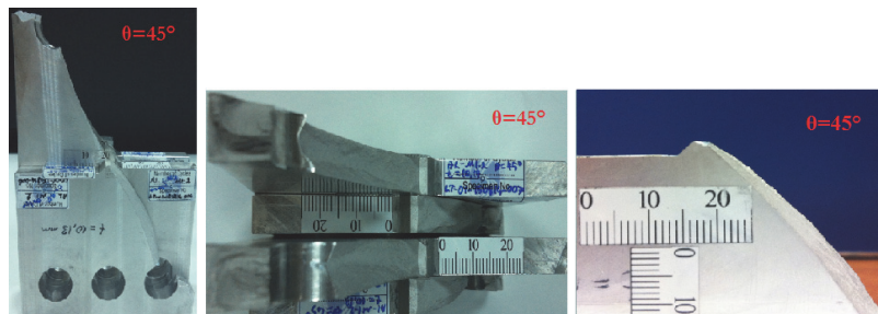
Figure 13: Overall broken sample pictures and fracture surfaces of CTS specimen for 45° loading angle.
