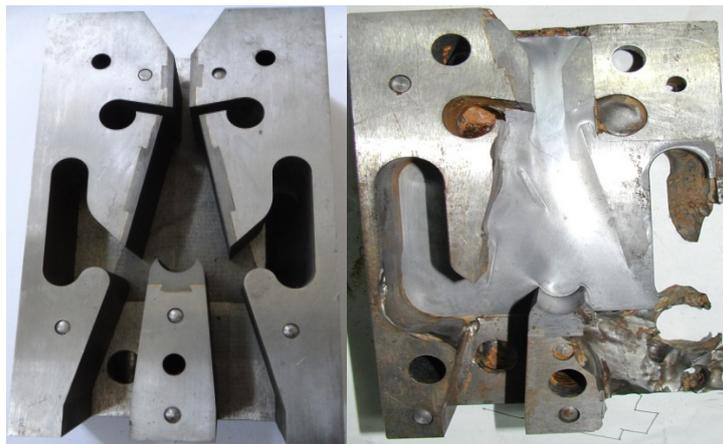
Figure 1: Failure of a fluidic amplifier before and after erosion by drilling muds.
