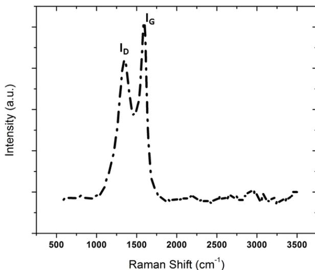
Figure 3: Raman spectrum of pyrolyzed bagasse fibers
