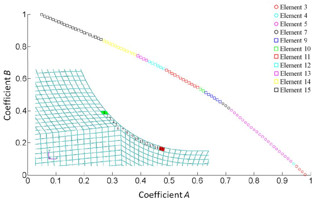
Figure 7: Limit curve that highlights elements that reaches the yield condition before others.
