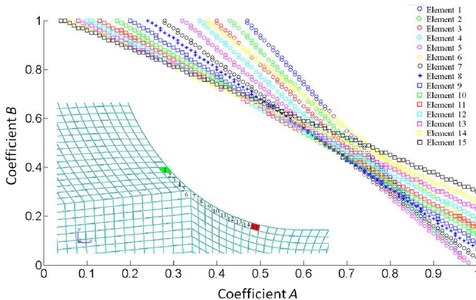
Figure 6: Combination of  $A$  and  $B$  and the relative most stresses element.
