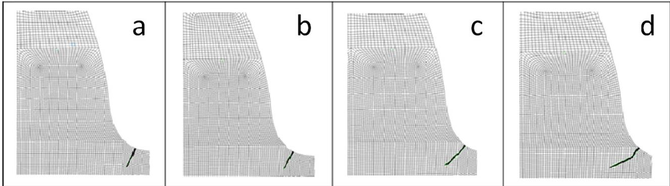
Figure 4: Interaction between bending and centrifugal load on the crack propagation direction: a) F + rotation; b) 2F + rotation; c) 5F + rotation; d) 8F + rotation.
