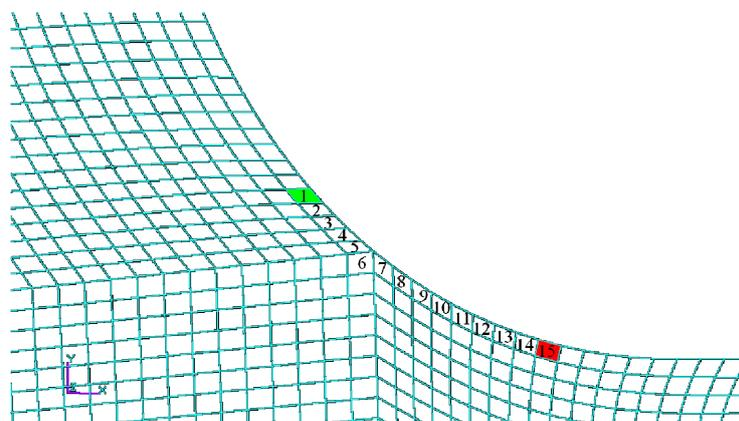
Figure 5: Elements where the yield stress is reached (green: only bending force applied, red: only centrifugal load applied).
