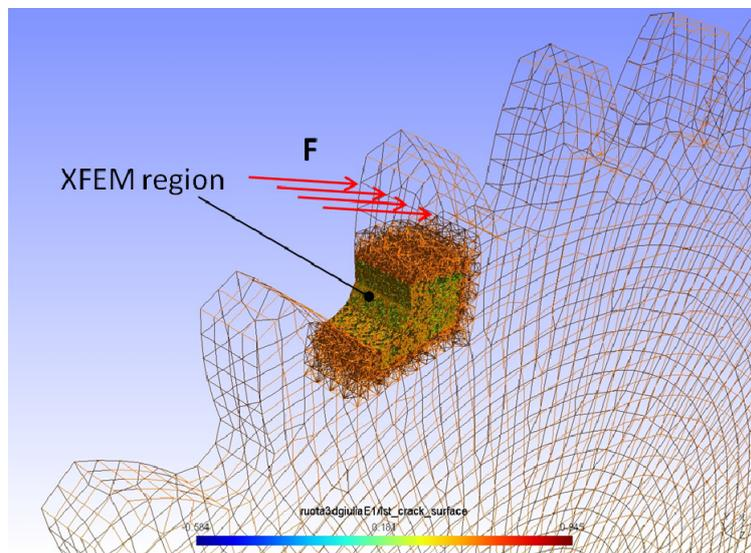
Figure 2: 3D extended finite element model (XFEM).
