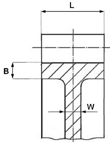
Figure 3: Geometric parameters of the wheel.
