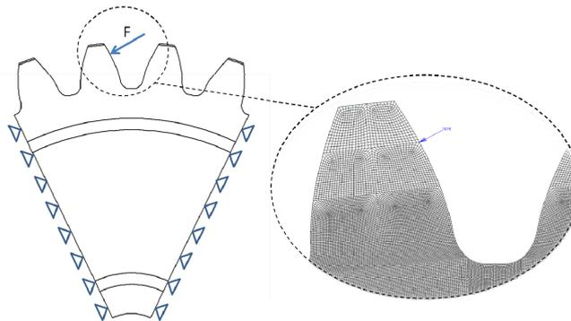
Figure 1: 2D finite elements model and mesh refinement.
