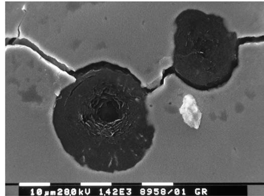
Figure 6: Graphite nodule – matrix debonding and graphite nodule internal damaging.
