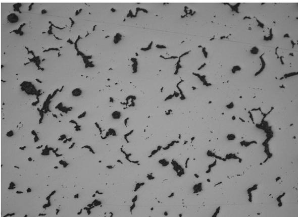
Figure 3: Defects in DCIs. Compacted graphite (x100). Courtesy of Zanardi Fonderie S.p.A.
