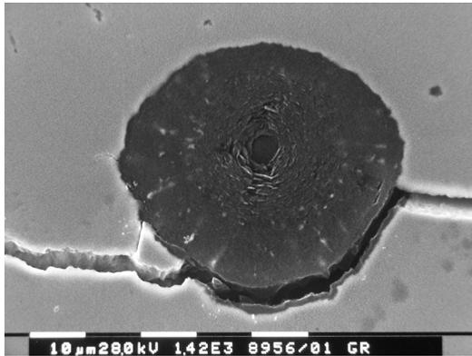
Figure 5: Graphite core-graphite-shield debonding (with residual graphite).
