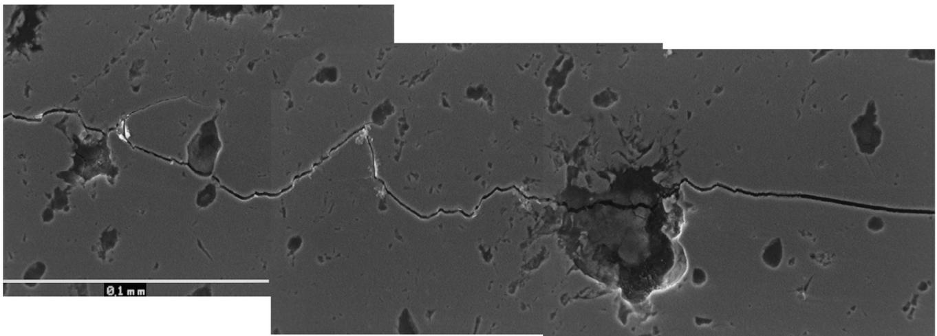
Figure 13: Ferritized DCI. Crack path.
