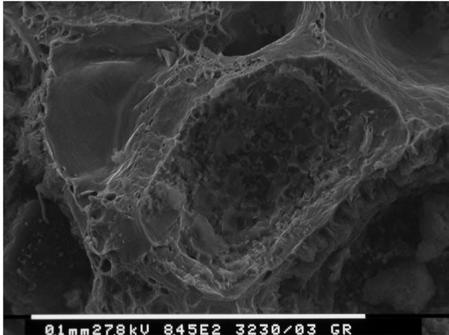
Figure 19: SEM observation of the fracture surface (after overloads).
