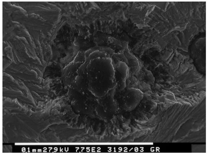
Figure 15: Ferritized DCI. SEM fracture surface analysis ( $\Delta K = 16 \text{ MPa}\sqrt{\text{m}}$ ).
