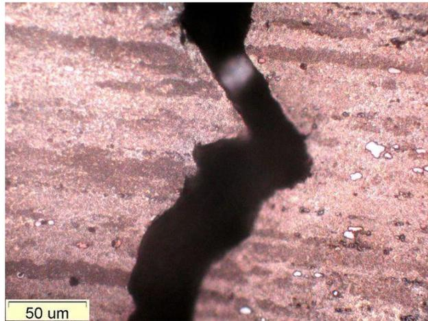
Figure 10: Fatigue crack path of the aluminium alloy 2024.
