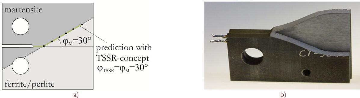
Figure 8: a) Gradation angle  $\varphi_M$  and theoretical kinking angle  $\varphi_{TSSR} = 30^\circ$  determined by TSSR-concept, b) experimentally determined kinking angle  $\varphi_0 \approx 23^\circ$
