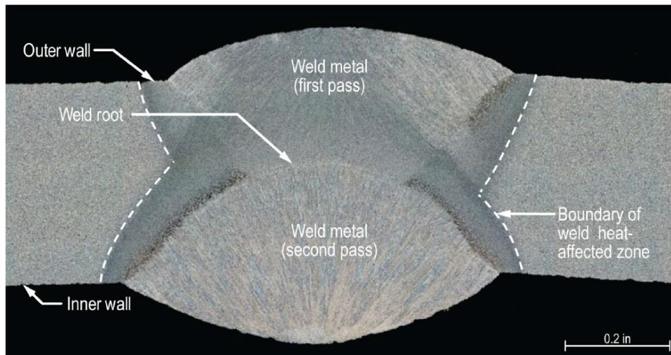
Figure 2: Metallographic cross section of a proper DSAW weld from NTSB Final Report, Fig. 19b.
