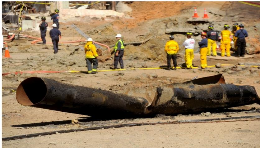
Figure 1: Photograph taken the day after the incident showing the ruptured segment of Line 132 that was ejected from the ground by the force of the rupture. Source: [www.dailyrepublic.com](http://www.dailyrepublic.com).
