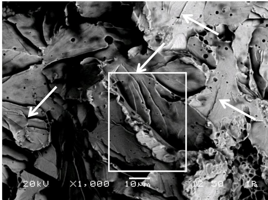
Figure 6: Exponent SEM image of brittle cleavage fracture morphology in Pup 1 final rupture zone. Representative river patterns associated with cleavage fracture are indicated by arrows.
