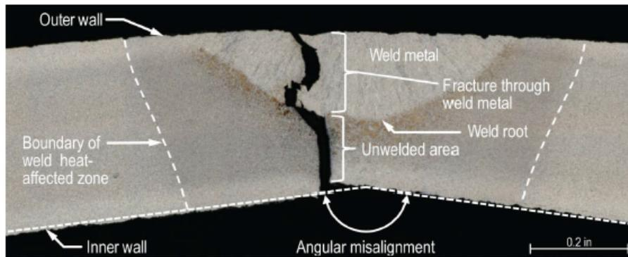
Figure 3: Metallographic image from NTSB Final Report (Fig. 19a) that shows the single-side weld in Pup 1.
