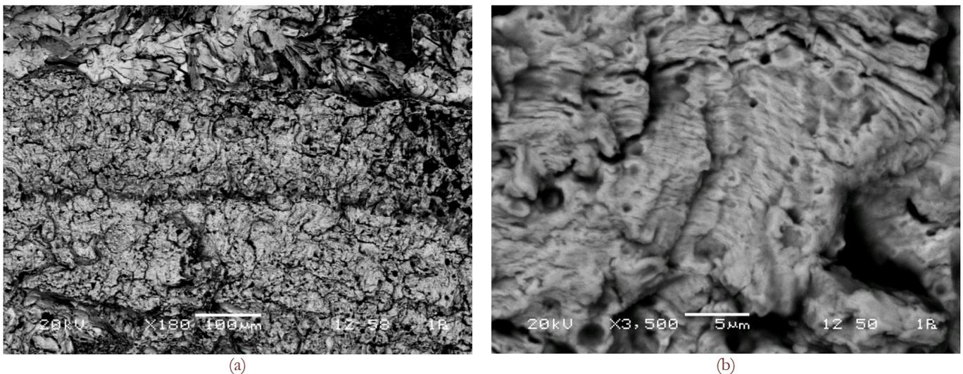
Figure 7: Exponent SEM images: (a) Fatigue striations were observed within Regions A & B, between the ductile tear (Region D) and the final brittle fracture (Region C); (b) Close-up of Region B in image (a), showing representative fatigue striations (within the box).
