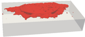
Defect B: 30° - Semi-elliptical
