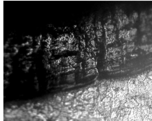
Figure 9: Micrographic analysis. Under site of scale surface. Discontinuous scale due to pronounced penetration. – 200 X.
