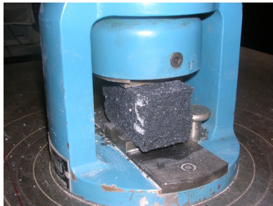
Figure 7: Compressive test on part of the sample coming from flexural test.
