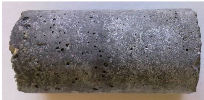
Figure 5: Mortar containing 5 wt% MWCNTs with respect to cement (cylinder is 4 cm in height and has a diameter of 2 cm).
