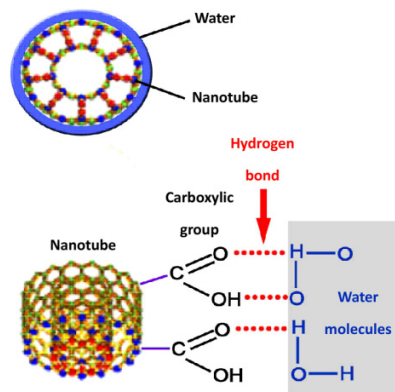
Figure 13: Possible interaction between COOH-MWCNTs and water molecules during cement hydration process [17].
