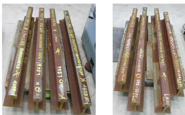
Figure 1: Rail sections from which specimens have been extracted.
