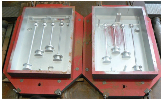
Figure 1: Wood model of the casting realised to evaluate the hot tearing behaviour of the alloys.
